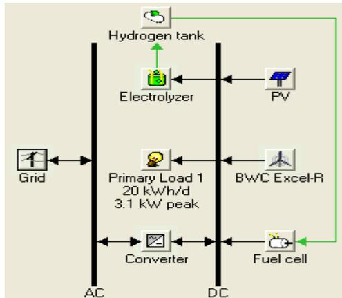
**Fig. 15. Grid connected PV-wind hydrogen power system components.**
