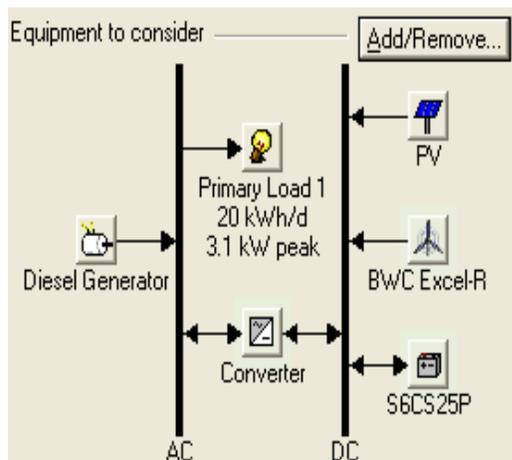
Fig. 6. PV-wind-diesel power system components.
