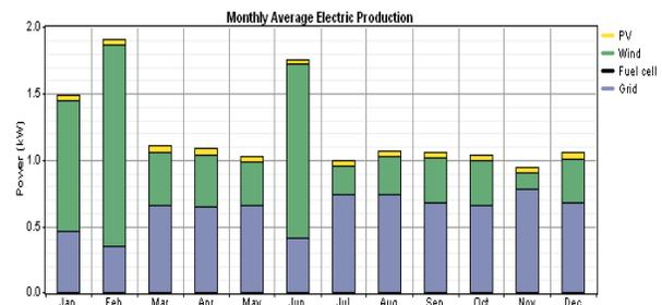
**Fig. 18. Monthly electricity production trend of the grid connected PV-wind-hydrogen system.**
