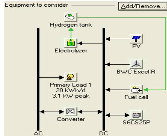
Fig. 10. Standalone PV-wind-hydrogen power system components.
