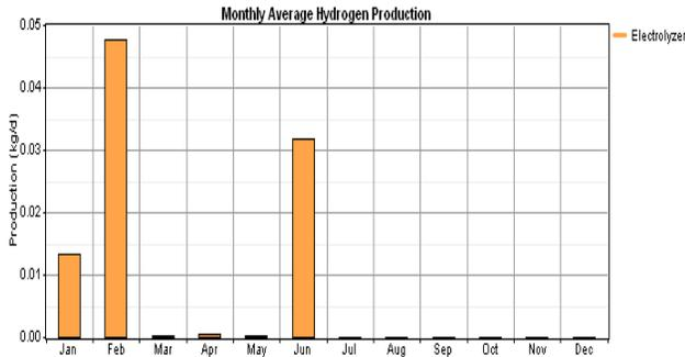
Fig. 19. Monthly hydrogen production for the grid connected PV-wind-hydrogen system.
