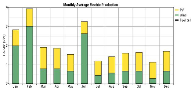
**Fig. 13. Monthly electricity production trend of the stand alone PV-wind-hydrogen system**
